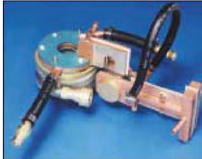
Fig. 1 — Magnetic flux concentrators for induction heating coils are made from high-permeability, low-power-loss materials. This scan inductor has flux concentrators (green rings) on top and bottom of a water-cooled single-turn copper coil. A quench ring is located below the bottom flux concentrator. Flux-trol Mfg. Inc., Auburn Hills, Mich, supplied the concentrators. Photo courtesy Inductoheat Inc., Madison Heights, Mich.
