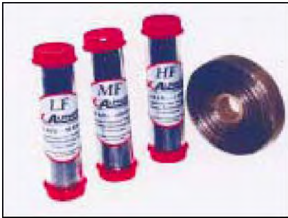
Fig. 5 — Some flux concentrator materials are supplied in a softened condition and can easily be formed into a shape sufficiently accurate for development purposes and subsequently machined, if desired, to exact tolerances. Photos of moldable Alphaform magnetic flux concentrator courtesy Alpha 1 Induction Service Center, Columbus, Ohio.
