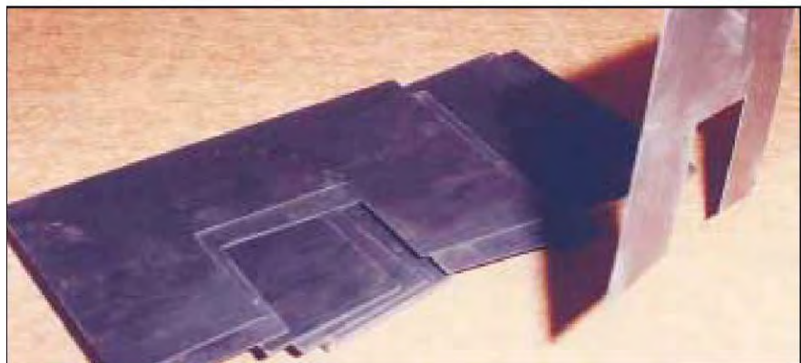
Fig. 4 — Laminations are among the materials used for flux concentrators. They are punched out of grain-oriented magnetic alloys, and stacks of them are used effectively from line frequency to 30 kHz. The typical lamination thickness range is 0.05 to 0.8 mm (0.002 to 0.03 in.).
