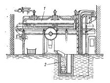
Fig. 3. Diagram of apparatus for heattreatment of forgings with utilization of forging heat. 1) Conveyor tempering furnace; 2) quenching tank.
