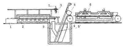
Fig. 2. Diagram of apparatus for quenching and tempering of forgings.
