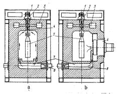
Fig. 5. Cross section of high-temperature (a) and low-temperature (b) overhead conveyor furnaces. 1) Overhead conveyor; 2) covered slots; 3) flue; 4) hanger; 5) forging; 6) device for recirculating combustion products; 7) combustion chamber; 8) burner. The apparatus replaces moving hearth furnaces that require four men working under severe conditions, who are exposed to the influence of radiant heat from forgings heated to 900°.
