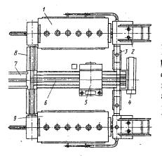
Fig. 1. Apparatus for heat treating forged turbine blades. 1) Pusher quenching furnace; 2) quenching device; 3) air spray; 4) belt conveyor; 5) washer; 6) intermediate conveying device; 7) loading station; 8) transporting device to feed forgings to furnace; 9) pusher tempering furnace.
